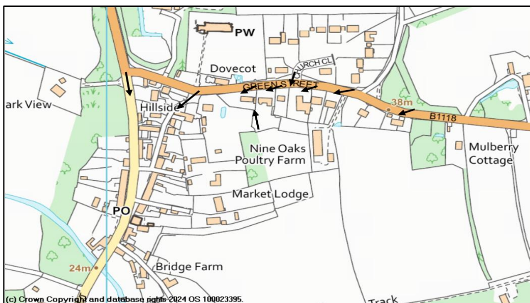
Figure 10. Approximate floodwater flow routes on Green Street
