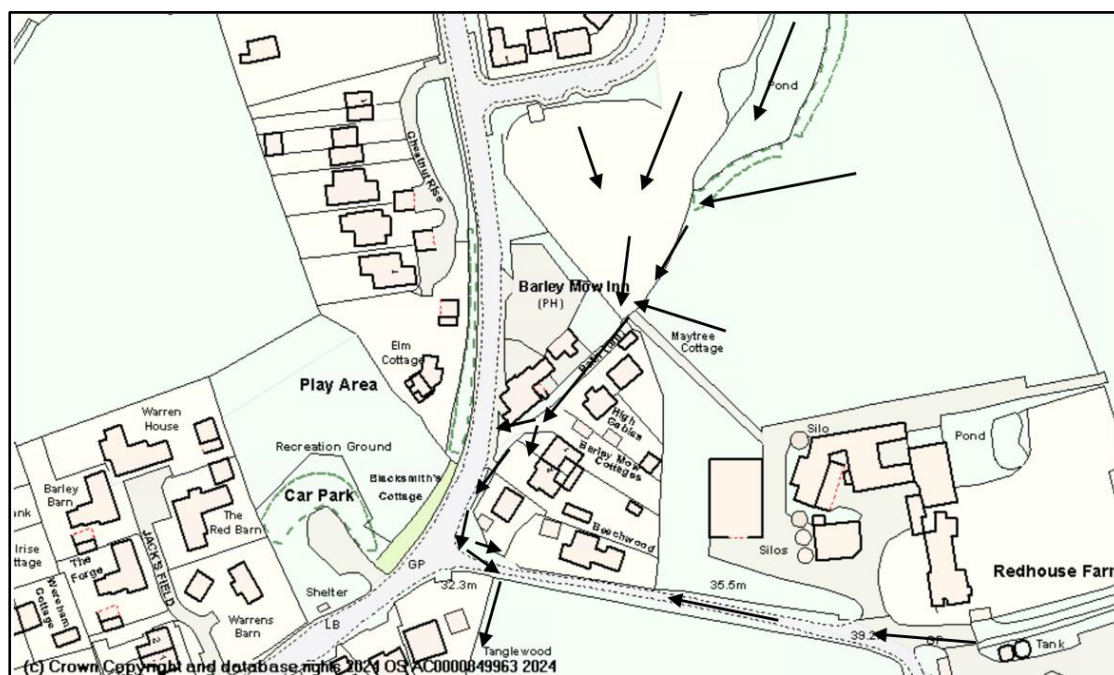
Figure 16. Approximate floodwater flow routes on Mow Hill
