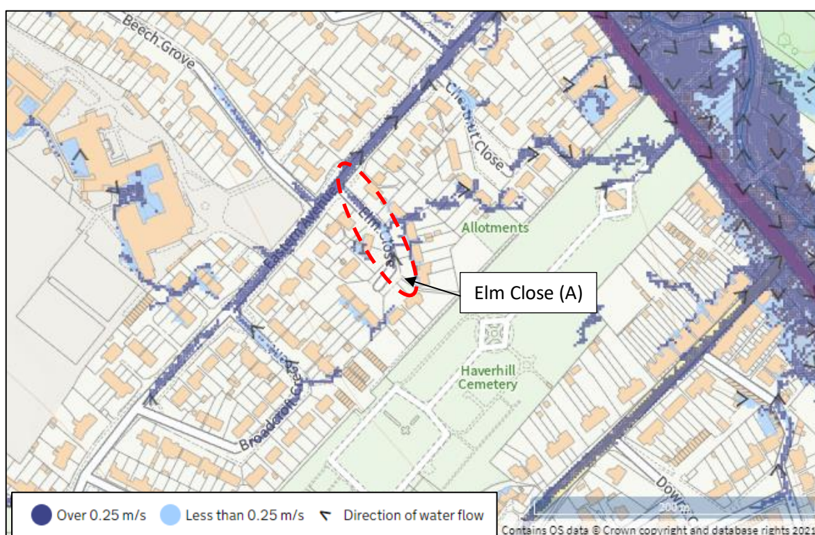
Figure 6 - Surface water flood risk: water velocity in low-risk scenario (GOV.UK mapping)
