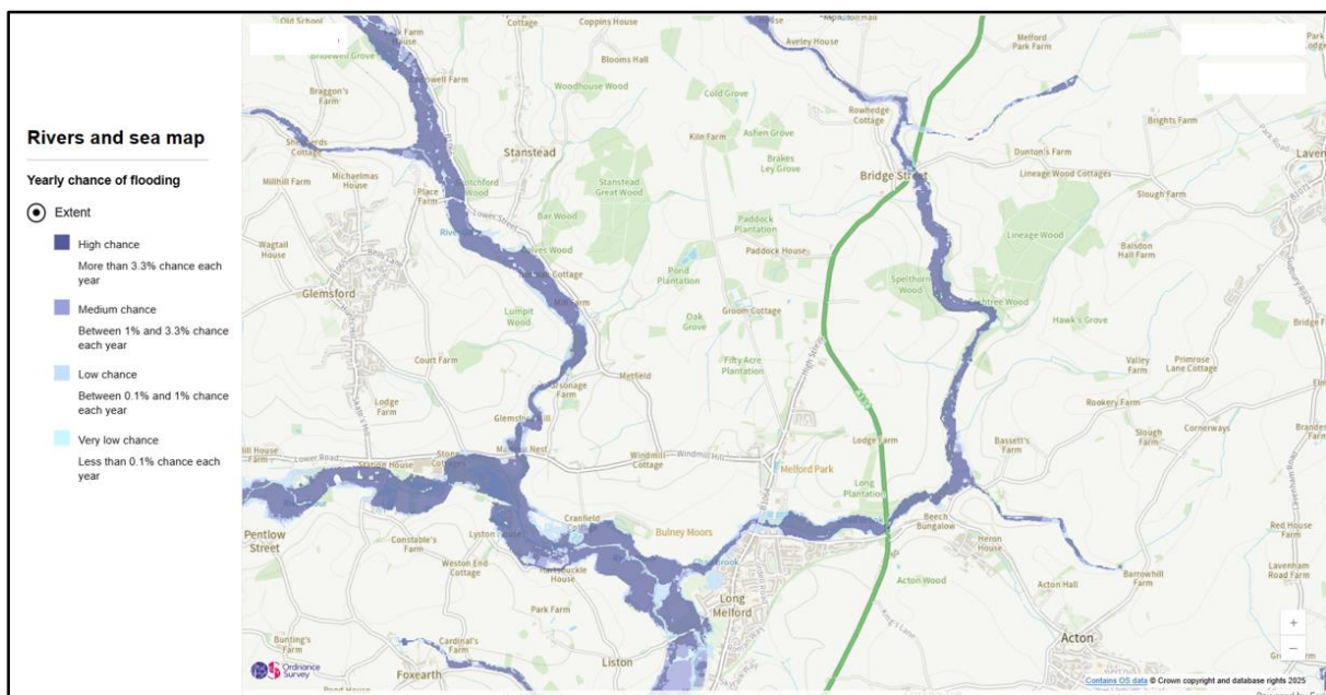
Figure 5. Predicted flood risk from river water (fluvial)
